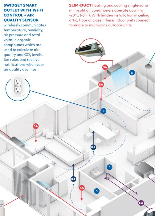
**MULTI-ZONE HEAT PUMP** is capable of delivering
