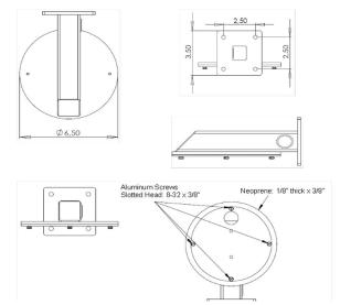
Note: Mounting hardware is included with all of the kits and mounting options listed in this document. Included hardware does not include fasteners or anchors for mounting to the wall itself.
