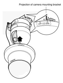
3 Turn this bracket clockwise until the projection of the camera mounting bracket aligns with "LOCK" of this bracket.
