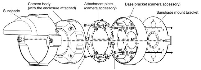
Fixing screws for attachment plate (x4, camera accessory)
