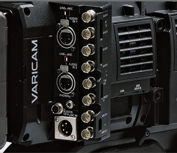
Side connector panel of the recorder
