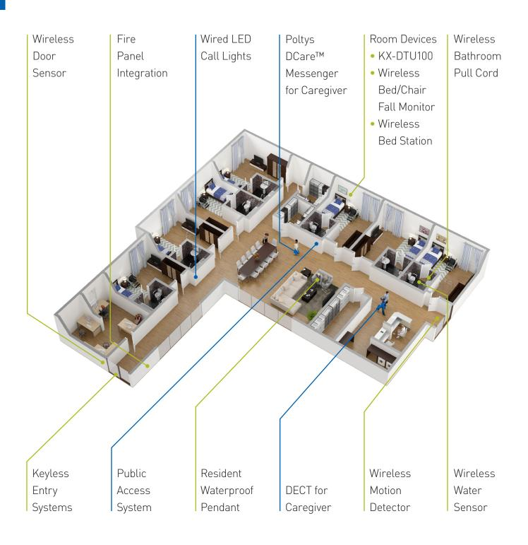
The Panasonic Nurse Call System can be customized for integration with building hardware and software systems such as door sensors and fire alarms or with databases.\* \*Some systems may not be compatible
