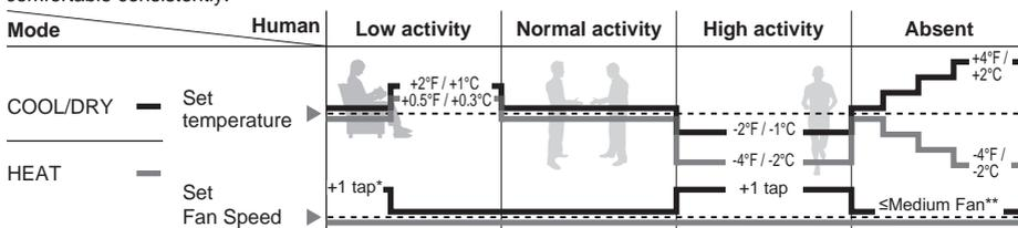
\* During low activity, fan speed 1 tap up for first 15 minutes or until set temperature is reached.
