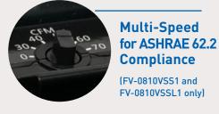
Multi-Speed for ASHRAE 62.2 Compliance allows you to select the proper CFM settings to satisfy ASHRAE 62.2 continuous ventilation requirements. The fan runs continuously at a preset lower level (0, 30-70, in 10 CFM increments), then elevates to a maximum level of operation (80 or 100 CFM) when the wall switch is turned on.
