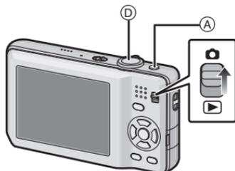
**1** Slide the [REC]/[PLAYBACK] selector switch to **[📷]**.
