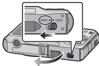
**2** **Battery:** Insert until it is locked by the lever **(A)** being careful about the direction you insert it. Pull the lever **(A)** in the direction of the arrow to remove the battery.
