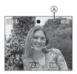
When the jitter alert appears, we recommend using a tripod. If you cannot use a tripod, be careful of how you hold the camera. (P31)
