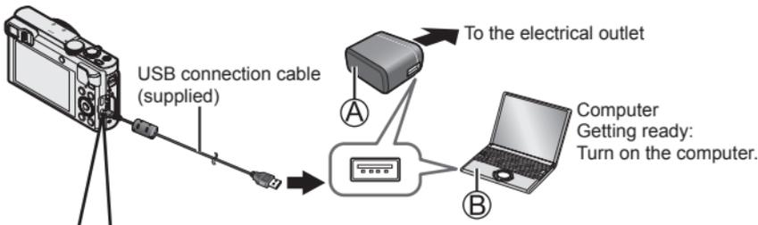
**When charging the camera, connect the USB connection cable (supplied) to the [AV OUT/DIGITAL] socket.**
