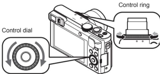
Items that can be set by the control ring/control dial vary depending on recording modes. Following are the pre-assigned settings.
