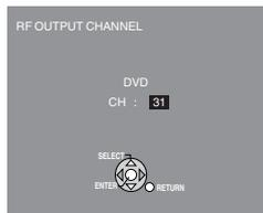
If you can't see the test pattern screen clearly, repeat step 1 and 2 to select RF output channel again.
