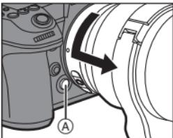
**2** While pressing the lens release button on the teleconverter **(B)**, rotate the teleconverter in the direction of the arrow until it stops and then remove it.
