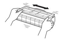
3 Detach the protective cover (③) from the toner cartridge, and remove the protective sheet (④) from the drum cartridge.
