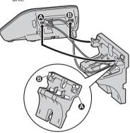
Adjust the adaptor to hold the base unit, then push it in the direction of the arrow until it clicks into place.
