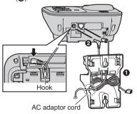
Insert the hooks on the wall mounting adaptor into holes (A) and (B) on the base
