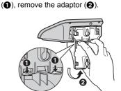
To remove the wall mounting adaptor
