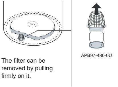
The filter can be removed by pulling firmly on it.
