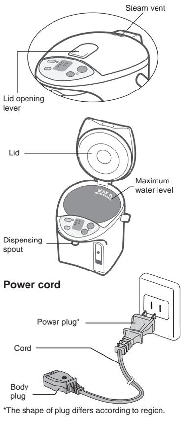
15. Do not allow small metal parts near the body plug.
