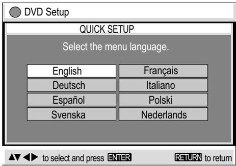
The navigator keys of the remote control unit allow you to move between menus and to accept or change the selected settings.
