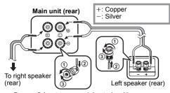
Be careful not to cross (short-circuit) or reverse the polarity of the speaker wires as doing so may damage the speakers.
